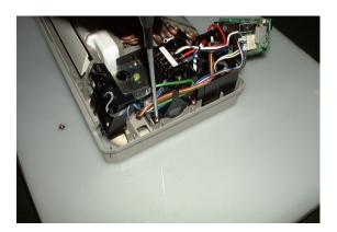
② Remove the connectors for sensor, fan motor and flap motor, which are connected to the electrical component box.
